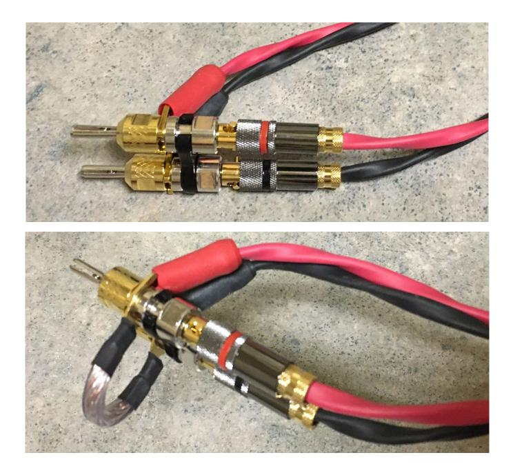
The test configuration allows a reliable and consistent termination. In-use would use the Cardas CABD banana and terminate the second cable spades onto the CABD as shown below. This removes a banana needed for the test set-up when we used locking banana on one cable end, versus the CABD, and spades on the opposite end.
