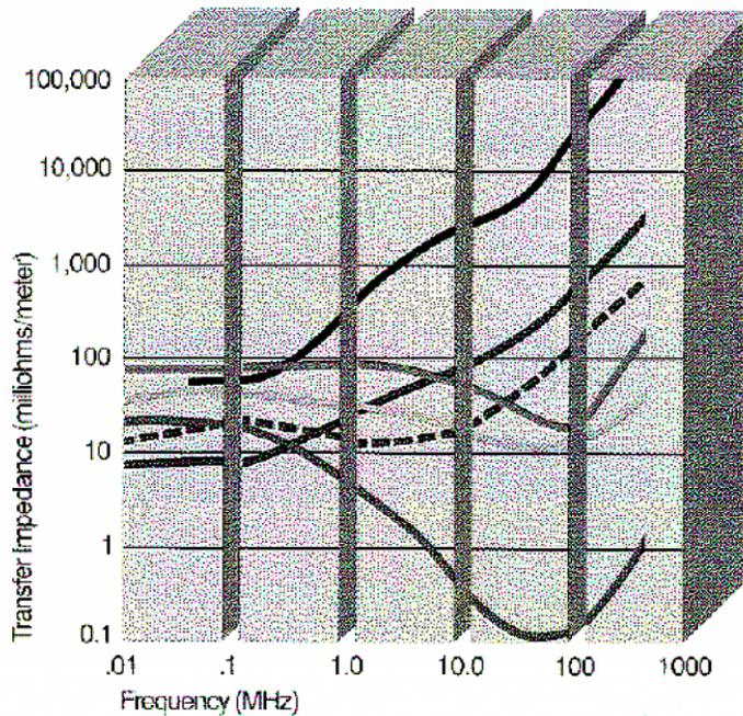
The lower the value of transfer impedance, the more effective the shielding.
