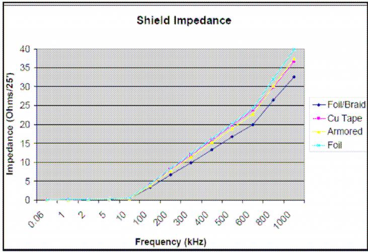
A SEED (Shield Effectiveness Evaluation Device per IEC 61196-1) test shows the dB relationship to a Lower Shield Impedance. Series number 5 with a 95% coverage 45-degree braid and Duofoil tape is clearly superior.
