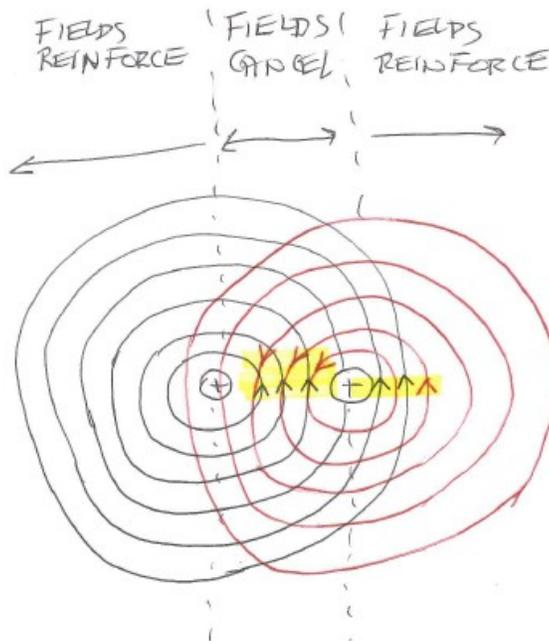
**OVERALL 1 X 4 WIRE CONDUCTORS ELECTROMAGNETIC SIGNAL FIELD CANCELLATION**
