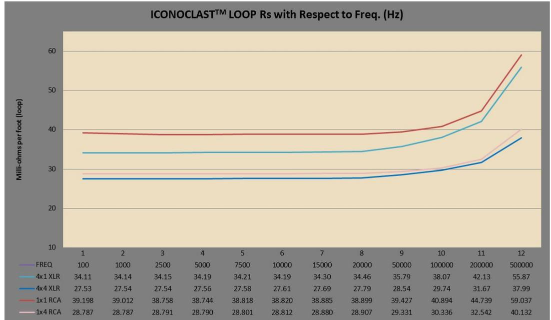
The RCA interconnect has also been updated with the new 1x4 (ONE wire made with FOUR conductors) design. The reactive variables will track with frequency like the single wire designs, but map to the altered L and C values.
