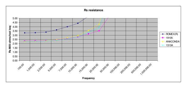
Below we look at what's in the wall, ROMEX, and the 19105. Are we a bottleneck to the wall supply? The data supports superior support from the wall with 19105 BAV cordage. We pass with less impedance at the low-frequency end yet offer better RF immunity at the high-frequency end.
