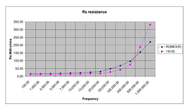
The Rs data above shows that the 19105 exceeds every option through the audio band. And the 19105 higher frequency Rs, even with a far larger AWG size, ramps up significantly, indicating a higher impedance assembly for passive EMI/RFI attenuation.
