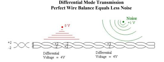
In the example above we show two wires, but the system is the same in a star quad. The signal we WANT is encoded as +2 volts and -2 volts. The noise can't "change its spots" relative the cable's twisted pairs and shows up as the same voltage on each wire, +1V noise in this example. The TWIST ratio helps make sure that the wires see the noise the same amount of time and this is vital to the function of the circuit.
