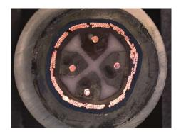
I could have used a cheaper and easier two wire XLR design but the inductive and signal coherence benefits of a star quad are too good to pass-up. If I can get the materials and quad design to achieve a high enough level of performance it is a better cable design.
