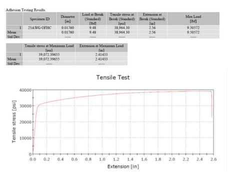
The 0.0176" diameter wire (0.0088" radius) is one half the diameters necessary for one full 18-mil skin depth at audio, so we have significantly improved current coherence through the wire @ 0.0176" diameter wire. Skin depth is FREQUENCY driven for a given material. The smaller the wire the larger the inner current magnitude will be relative to the surface current. We want as good a shot of that as we can get.
