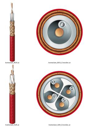
In the coaxial cable, the center of the wire to the inside of the tube is 0.098" / 2 = .049". Ok, so what? This is what. The capacitance is a squared law property and predominantly sees the ground closest to the wire. The shield on the opposite side of the XLR cable, to a first approximation, falls a way. We actually measure the capacitance BETWEEN the two cross paired wires but the ground location still influences the capacitance. Also, we have four wires that are capacitors.
