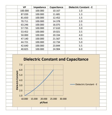
What does the cable actually measure on capacitance? The chart below shows 11.767 pF/foot. Notice that the capacitance values between each of any two wires has to be  $\sim 5$  pF/foot to "double-up" the two wires capacitance and still to arrive at a final  $\sim 11$  pF/foot! Yep, that's LOW capacitance. Capacitance adds in parallel so this is a significant issue when a design uses four wires.
