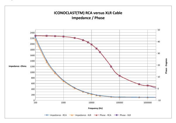
What we see above is impedance / phase for the XLR and RCA superimposed one on top the other. Note that there are four separate lines. We have two identical cables with exceptional reactive variables.
