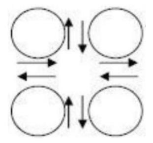
Where the arrows are OPPPOSITE each other in direction between any two wires, the field lines cancel. ACROSS from any TWO wires we also induce field cancellation with a star
