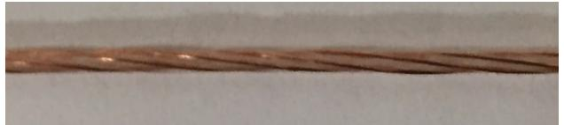
Technically, four -wire per conductor will increase capacitance some as we have more wires parallel to a dielectric, but the current coherence improves substantially, time aligning the low to high frequencies.
