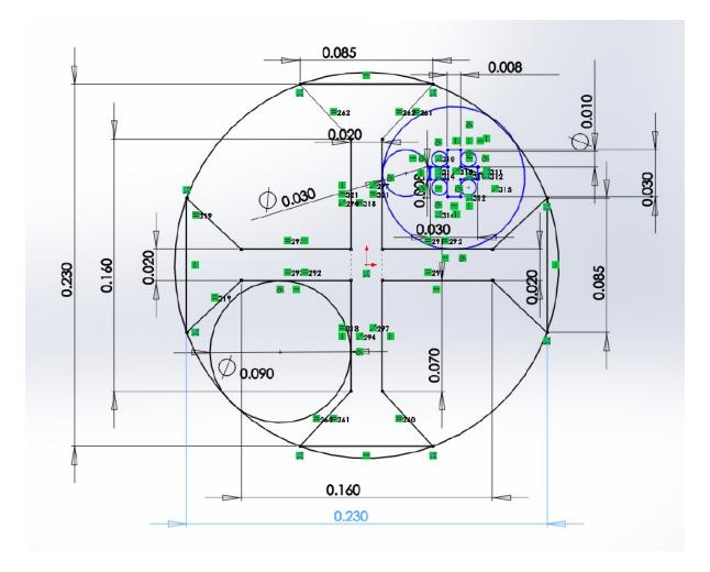
The X-filler is FEP, as would the 30-mil beading wrapped around the QUAD wire to lower the dielectric nearest the wire where it is most critical. The material issues all control capacitance, not inductance.
