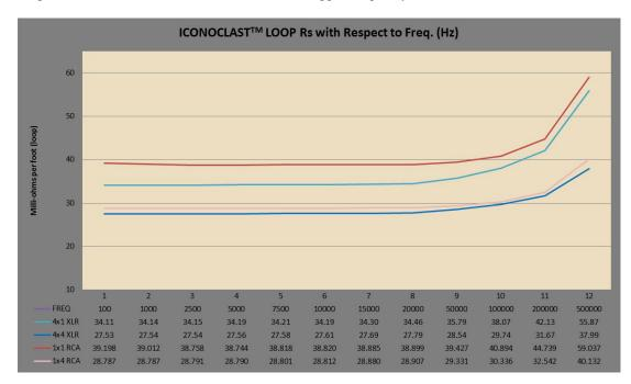
The RCA interconnect has also been updated with the new 1x4 (ONE wire made with FOUR conductors) design. The reactive variables will track with frequency like the single wire designs, but map to the altered L and C values.
