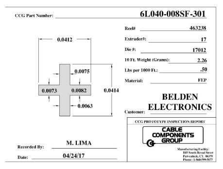
The overall belt is solid FEP, with a 36 AWG BC braid and a drain wire. A final solid FEP jacket finished the cable.
